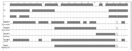
Fig.2-2 Time Diagram of Box Bending Mode
